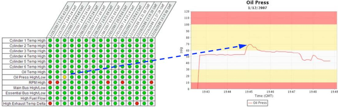
**Example of Remote Engine Monitoring System: OpenAero: a web-based maintenance and remote engine diagnostics application.**
