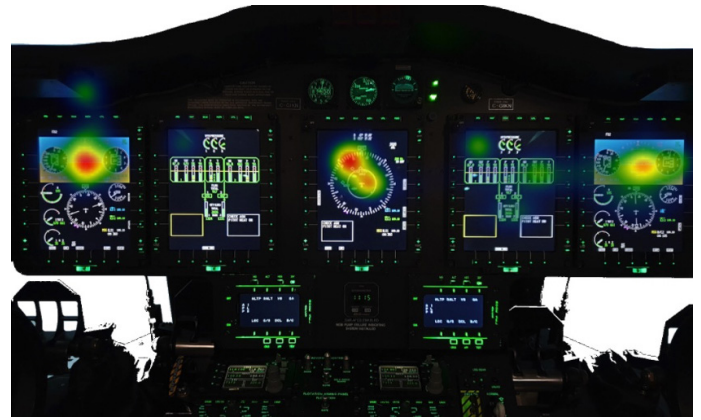
Figure 5. Heatmap showing the amount of looking in the first 15 seconds following an event onset (in this case a non-emergency technical failure). PF is on the left, PM is on the right. This is representative of a crew using the experimental mitigation. The attention to the aviate task is clear, as is the extra navigational monitoring by each pilot.
