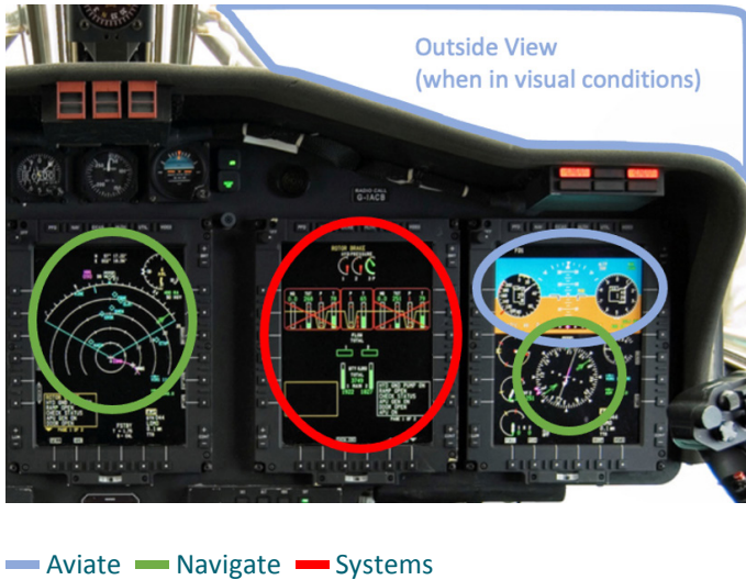
Figure 1: Simplified diagram showing the main screens for aviate, navigate and systems information in the S-92 helicopter. The research used more complex and complete mapping.
